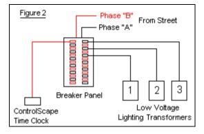
Figure 2 is the same simple setup as Figure 1, EXCEPT the Time Clock is now plugged into the "B" Phase. How will the signal travel from the "B" to the "A" Phase? Without a Phase Coupler, it will need to travel out to the
