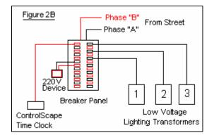
There are many times when there is a 220V device in the house, such as a dryer, oven, etc., that provides phase coupling for you. You just plug in, test signal, ...looks good, away you go.
