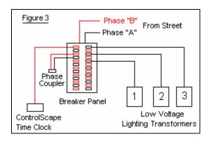
In Figure 3, a Phase Coupler is inserted. The signal no longer needs to travel out to the street to find the other Phase. It simply joins at the Phase Coupler.
