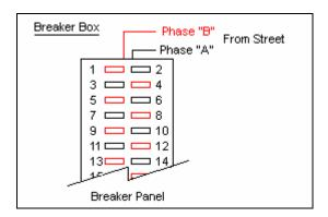
This may seem fundamental to some, but it is critical to understanding Phase Coupling. The diagram to the left shows a portion of a breaker box. The breakers in Red are on the "B" Phase and the breakers in Black are on "A". All panels are the same. Every other breaker in each column is on the same phase. For example, in the left column, breakers 1, 5, 9, 13.... are on the same phase. This is evident from a 220 breaker, which takes up two consecutive spaces so to get power from both phases.
