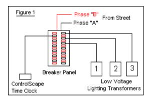
In Figure 1, there is a single panel. The two phases from the street are illustrated in Black and Red. In this scenario, all devices, including the Time Clock, are connected to the "A" Phase (Black). Clearly, the use of a Phase Coupler would not be required.
